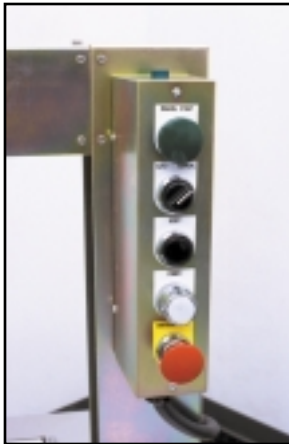
Magnetic Control Box
