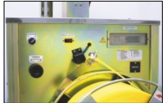
PLC Control with Diagnostics, Waist High Strap Loading, Maintenance Counter
